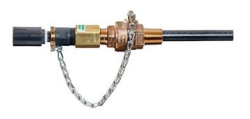
When injecting chemical solutions into process pipes, it is advisable to introduce the chemical into the process flow away from the wall of the process pipe, in order to minimize chemical attach or chemical deposits on the wall of the pipe and to improve rapid dilution / mixing.
